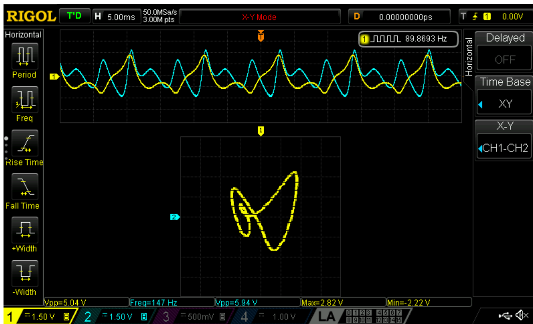
Figure 22: Phase Plane-Trajectory of x(t) vs. z(t) , A = 1.85V
