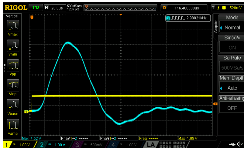
Figure 20: Unit-Impulse Response of 4th-Order Butterworth Filter, pt.1
