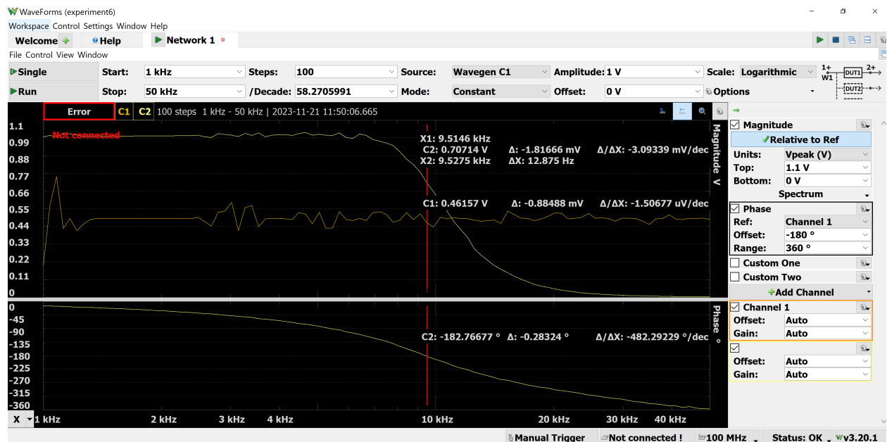
Figure 22: Magnitude, Phase Plot of 4th-Order Butterworth Circuit
